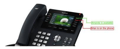
This manual is designed to guide customers through setting up the BLF (Busy Light Function) feature on compatible Yealink phones. The guide will presume you have already configured the VoIP registration settings. If you still need to register the phone to Montec Connect, please check the Setup Guides page or call Montec Connect on 1300 011 585.
